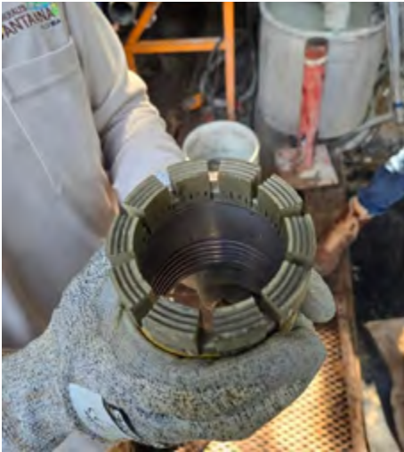
This is what a diamond drill bit looks like. Those blades you see are actually made of diamonds, what is the best material to cut through the ground and retrieve the drill core. As I outlined in Paydirt page 120 , results from diamond drilling are the most reliable and considered the "final test."
