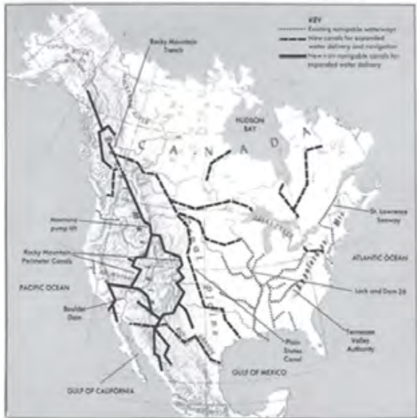
The NAWAPA Plan for Bringing Additional Fresh Water to the United States, Canada, and Mexico
