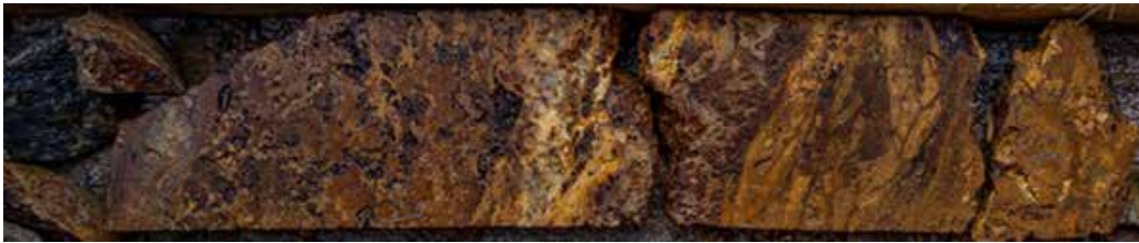
Drill core from hole SR20-29 – Textural example of high-grade gold mineralization present within the Domino zone – sample above graded 19.9 g/t gold and 71.6 g/t silver over 0.94 metres. The host felsic volcanic rocks are cut by an oxidized, vuggy, sheared quartz vein with intense limonite alteration. All primary textures have been destroyed by strain and alteration. Thin bands of chlorite and sericite trend along shear fabric. Shear contains ~15% pyrite and ~5% pyrrhotite. The length of the image is ~30 cm.
