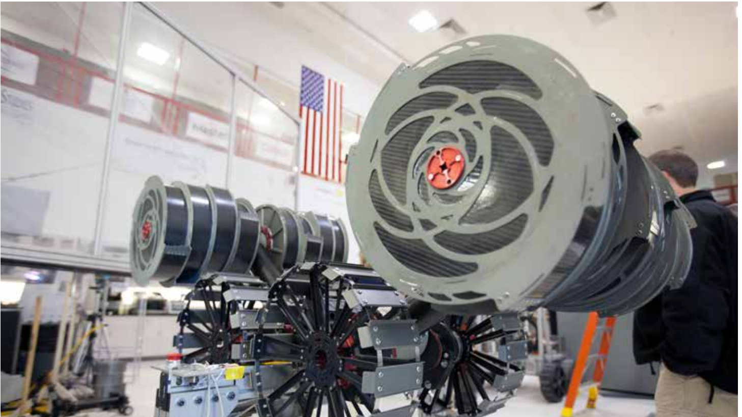
NASA's Regolith Advanced Surface Systems Operations Robot 2.0 (RASSOR, pronounced "razor"), shown here in Kennedy Space Center's Swamp Works, has several upgraded features that include being nearly half the weight of its predecessor and the ability to collect nearly three time more material and to operate autonomously. RASSOR 2.0 is one of NASA's robots designed to excavate material from other planets, a critical aspect of NASA's deep-space travel plans. For more information, go to go.nasa.gov/1RtcRES . Photo credit: NASA/Bill White
